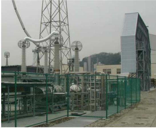
Fig.3. Terminals for 500-m cable tests
