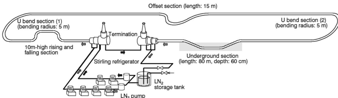
Fig.2. Schematic view of the layout of 500-m HTS power cable test system.
