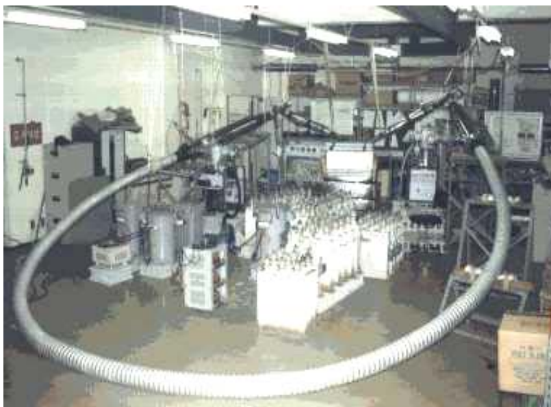
Development of extruded polymer insulated low temperature superconducting cable in Toyohashi University of Technology
