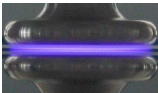
Fig.7 OAUGDP in a 1mm air gap at 11.93kHz 1762.5V
