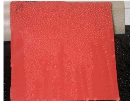
Fig.5 Hydrophobicity Test of RTV
