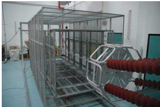
Fig.3 Corona cage used in the experiment
