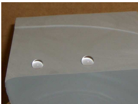
Fig.1 Water droplets set on a cut surface of SHCEP
