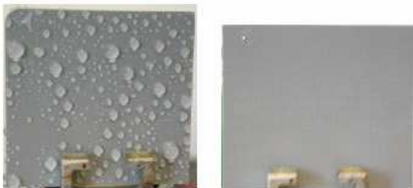
Fig.2 Spray test before (left) and immediate after (right) plasma-treatment shows that the plasma is effective to destroy hydrophobicity (fully wetted surface)
