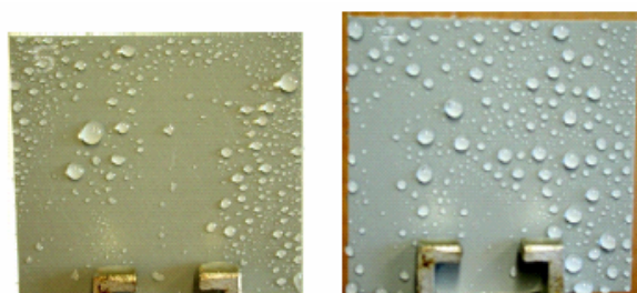
Fig.3 Spray test one day (left) and three days (right) after plasma-treatment shows hydrophobicity recovery after forced loss
