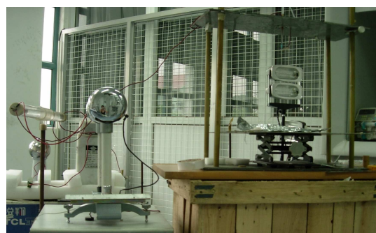
Fig.9 Experiment circuit of electro-spinning
