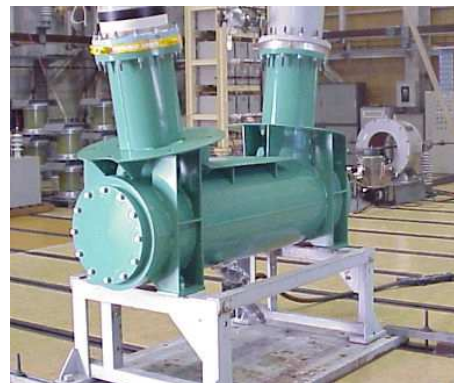
Fig. 2. View of the 72 kV-class CO 2 -GCB model (for single phase).
