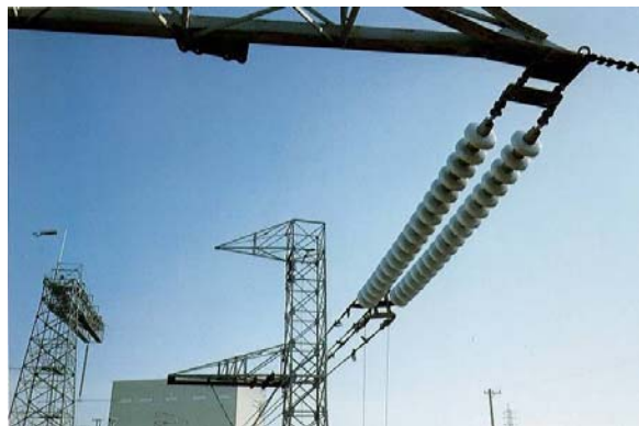
Artificial galloping test of tension insulator assembly
