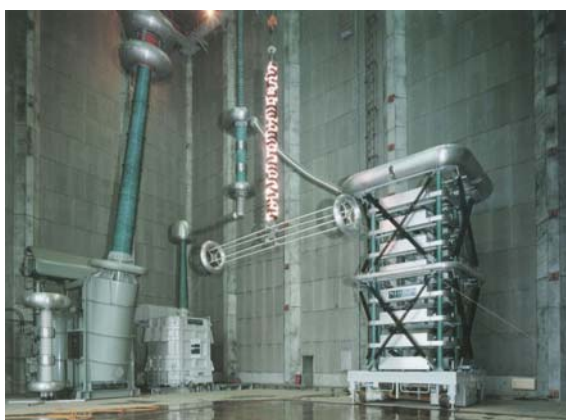
DC contamination test of DC500kV insulator assembly
