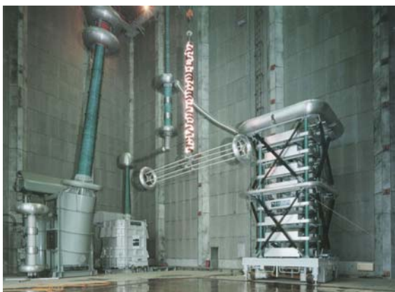
DC contamination test of DC500kV insulator assembly
