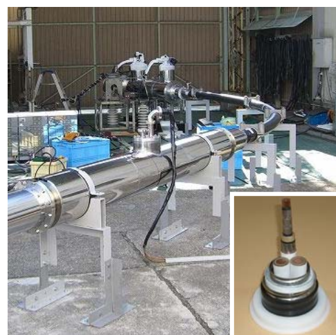
Fig. YBCO HTS cable cut model and photograph of the short circuit current test. The test cable was constructed of a 10m YBCO HTS cable and a cable intermediate joint.
