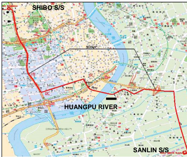
500kV SHIBO CIRCUIT ROUTE LAYOUT
