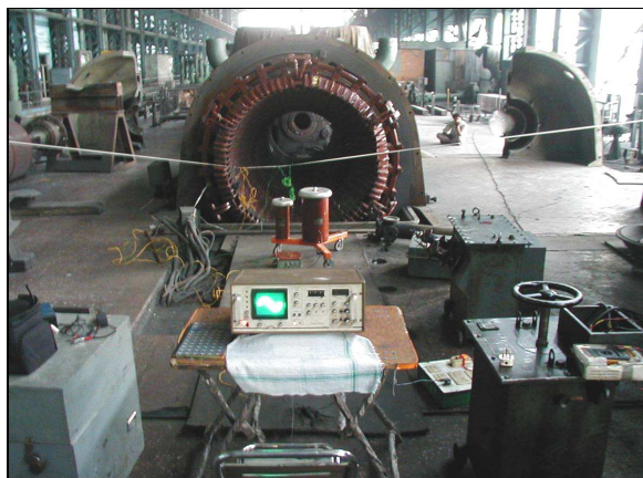
Figure 3: Diagnostic PD test on 110MW Turbo generator
