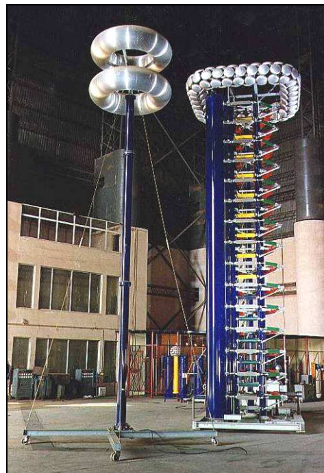
Figure 1: Impulse Voltage Generator, Bangalore
