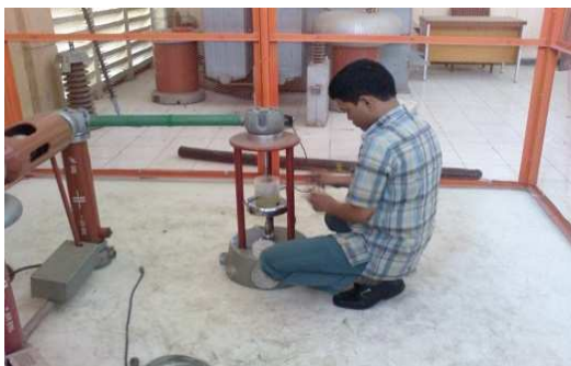
Figure 5: Conductivity Measuring Device for Oil Insulator
