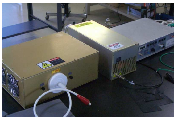
Fig. 1 Highly repetitive compact pulsed power generator for industrial applications.
