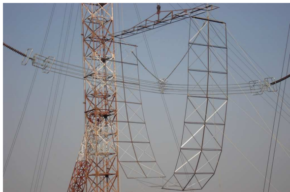
Figure 5: Testing under progress to optimize tower window clearance of 1200 kV ac line
