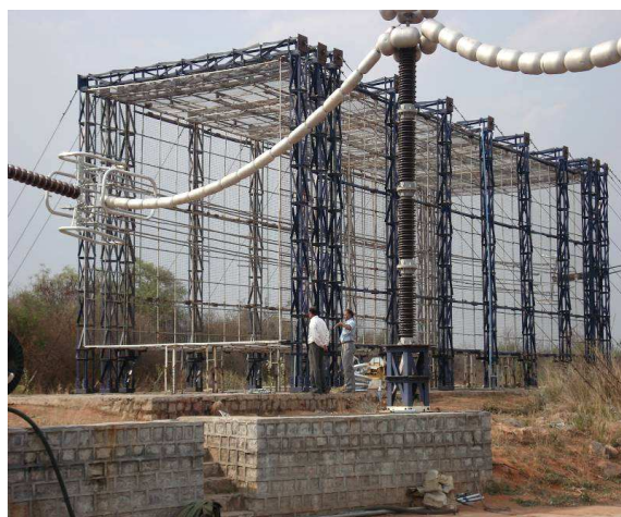
Figure 6: Corona cage with bundle conductor strung inside.
