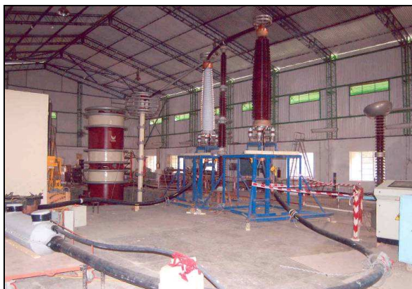
Figure 2: Testing of 220kV Cable
