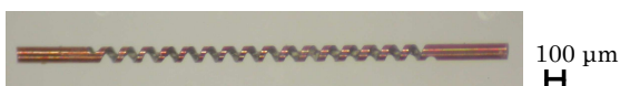
Fig.3 Micro-coil obtained by etching the specimen shown in Fig. 2. It was etched in ferric chloride solution.
