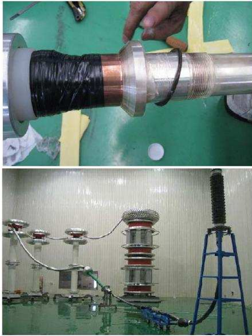
Figure 5: PD detecting sensor assembling and laboratory PD test for 110 kV XLPE cable (supported by Tianjin Electric Power Corporation).
