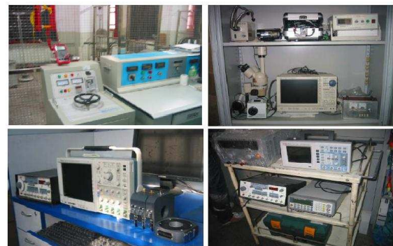
Figure 4: Devices for research of partial discharge measurement for XLPE power cable.
