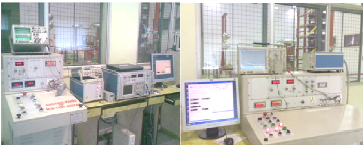
Figure 3: ICT enabled operation of AC & Impulse High voltage test system
