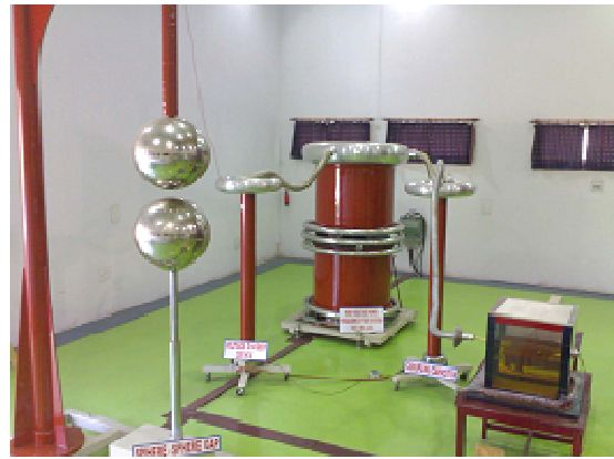
Figure. 4 A photograph of the schematic experimental setup of partial discharge measurement
