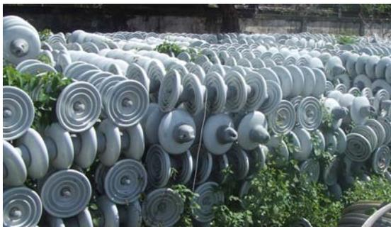
Figure 5 Large number of SCG Insulators removed from system
