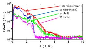
Fig. 4 THz intensity spectra and standard deviations of reference and sample.
