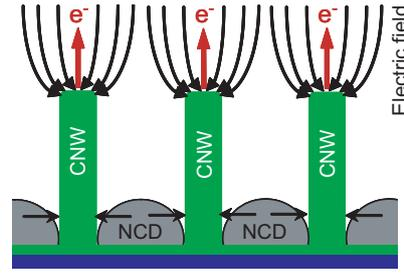
Schematic of CNW/NCD emitter
