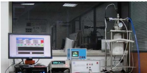
Figure 5. TSC measurement system
