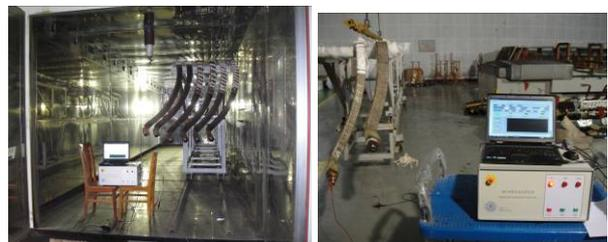
Figure 7. Diagnosis of motor bar using IRC 3.0 system
