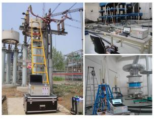
Figure 6. Diagnosis of XLPE cable using IRC 3.0 system
