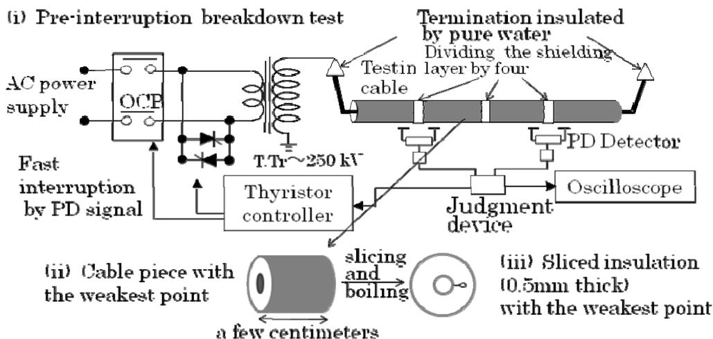
Fig.1 Pre-interruption breakdown test and investigation of the water-tree
