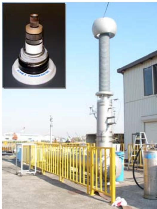
Fig. 275kV HTS power cable cut model and outdoor termination.
