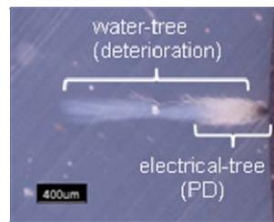
Fig.4 Water-tree and electrical-tree
