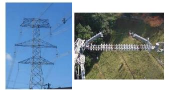
Fig. 4 Test Situation of Galloping Simulation Test
