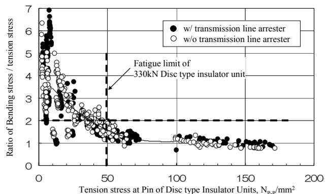
Fig. 5 Stress on Pin of Disc type Insulator Units
