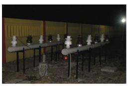
Figure 7 Silicone-coated insulators at Pangandaran substation testing site
