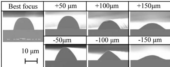
Fig. 1 Various profiles obtained by changing focal position. Wavelength and exposure time were fixed at 405 nm and 8 min. Plus defocus means that the wafer is placed far from the lens.
