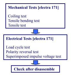
Fig. 1 Procedure of type test used in this project
