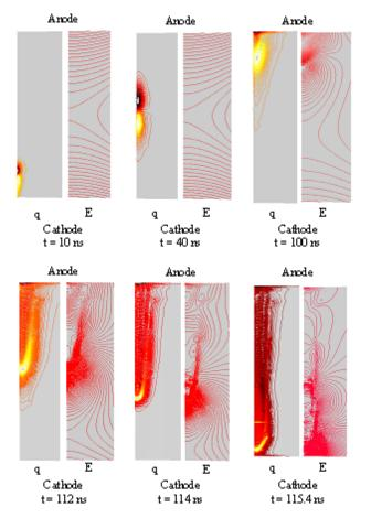
**Figure 2:** Propagation of streamer (q) and electric field distribution (E) at various times between the sphere gap
