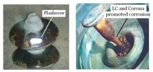
Figure 1 Insulator failure (a) flash over (b) mechanical failure
