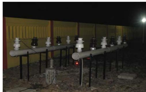
Figure 7 Silicone-coated insulators at Pangandaran substation testing site
