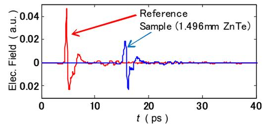
Fig. 3 THz electric-field pulse waveforms measured with a THz-TDS.
