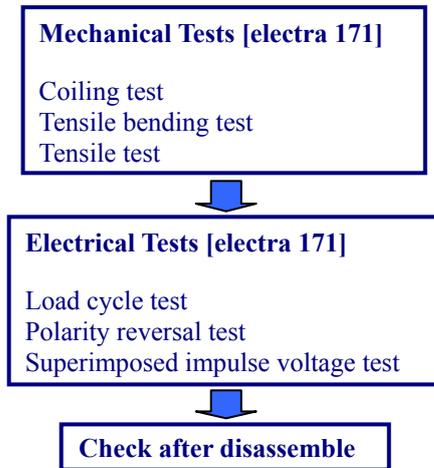
Fig. 1 Procedure of type test used in this project
