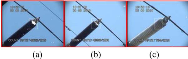
Figure 9 Corona intensity at uncoated (a), (b) and coated (c) insulators measured using UV Camera
