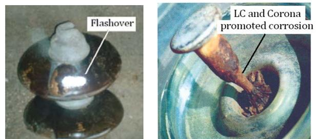
Figure 1 Insulator failure
