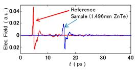
Fig. 3 THz electric-field pulse waveforms measured with a THz-TDS.
