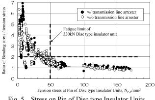
Fig. 5 Stress on Pin of Disc type Insulator Units
