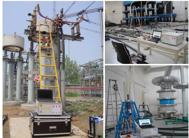
Figure 6. Diagnosis of XLPE cable using IRC 3.0 system
