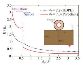
**Figure 3:** Field distribution in configuration of a covered conductor on a spacer for different spacer materials
