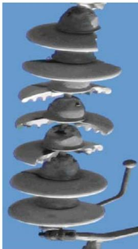
Figure 4 Broken string SCG insulator
