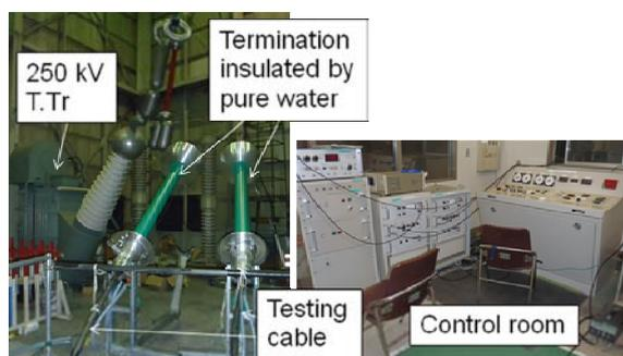
Fig.2 Facilities of pre-interruption breakdown test
