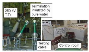
Fig.2 Facilities of pre-interruption breakdown test
