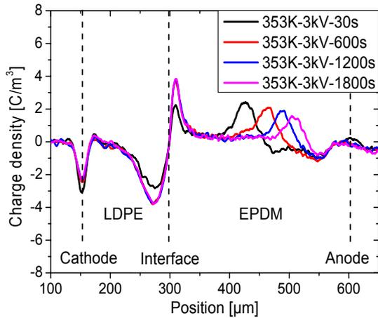
Figure 3. Space charge at the interface between the insulation of cable and its accessory
