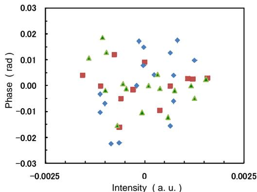
Fig. 5 Correlation of random errors in between phase and intensity spectra at 1.20 – 1.37 THz in frequency domain.
