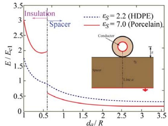
**Figure 3:** Field distribution in configuration of a covered conductor on a spacer for different spacer materials
