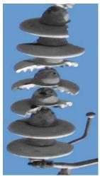
Figure 4 Broken string SCG insulator
