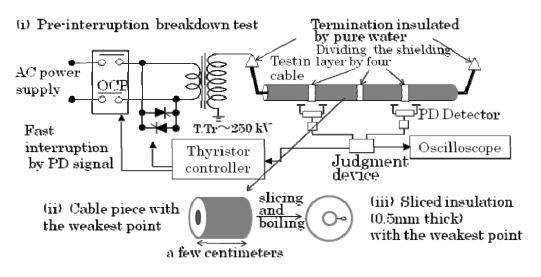
Fig. 1 Pre-interruption breakdown test and investigation of the water-tree
