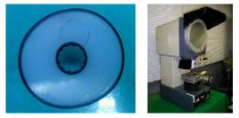
Fig.3 Sliced insulation and magnifying glass
