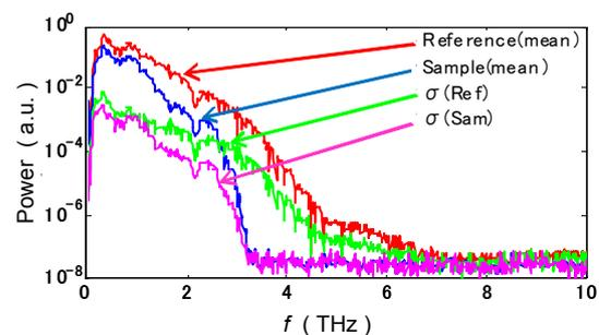
Fig. 4 THz intensity spectra and standard deviations of reference and sample.
