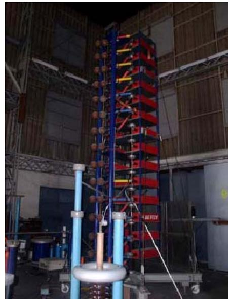
**Figure 1:** 1400kV impulse voltage generator
