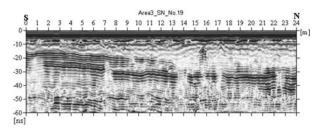
Fig. 2. Example of Cross Sectional Diagram obtained at Shikiryou Archaeological Site
