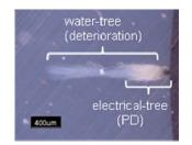
Fig.4 Water-tree and electrical-tree
