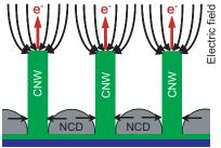
Schematic of CNW/NCD emitter
