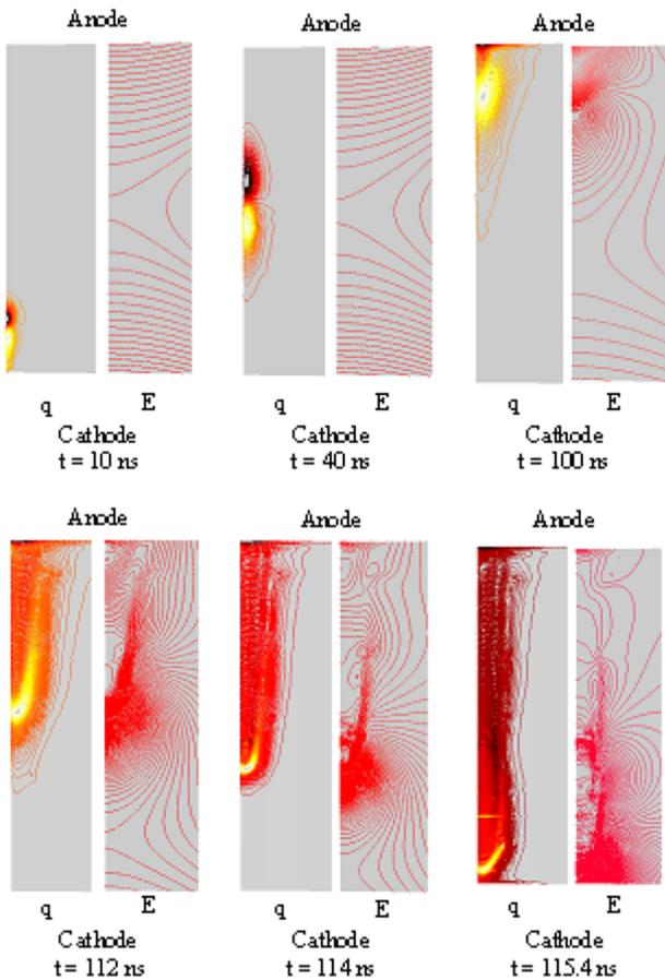
**Figure 2:** Propagation of streamer (q) and electric field distribution (E) at various times between the sphere gap
