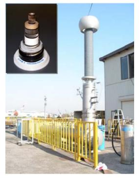
Fig. 275kV HTS power cable cut model and outdoor termination.
