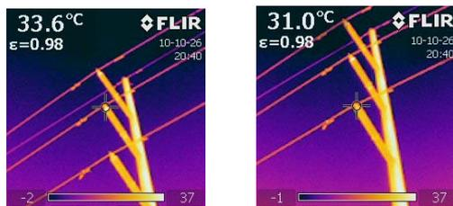
Figure 10 Thermal image of insulator (a) phase S (uncoated) and (b) phase T (coated)
