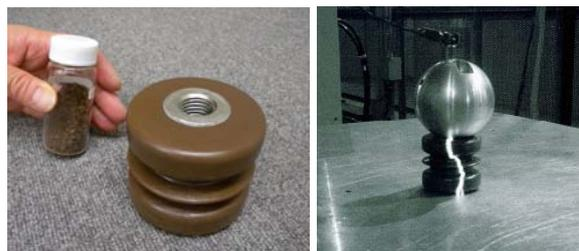
Figure The lignocellulose powder, polymer insulator (left) and appearance of examination (right).
