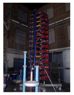
Figure 1: 1400kV impulse voltage generator
