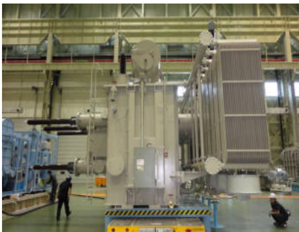
Figure 4. 80kV HVDC Transformer (LS Industry)
