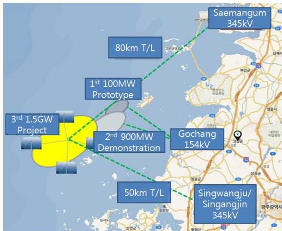
Figure 3. HVDC T/L Project in Off-Shore
