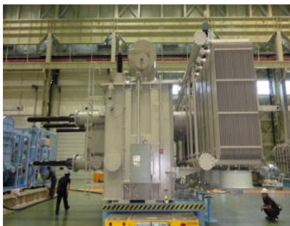
Figure 4. 80kV HVDC Transformer (LS Industry)
