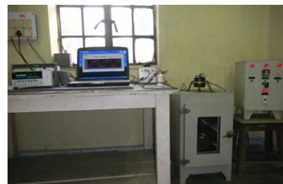
Fig. 4.4.2.1 Experimental set-up for FDS using non-sinusoidal excitation
