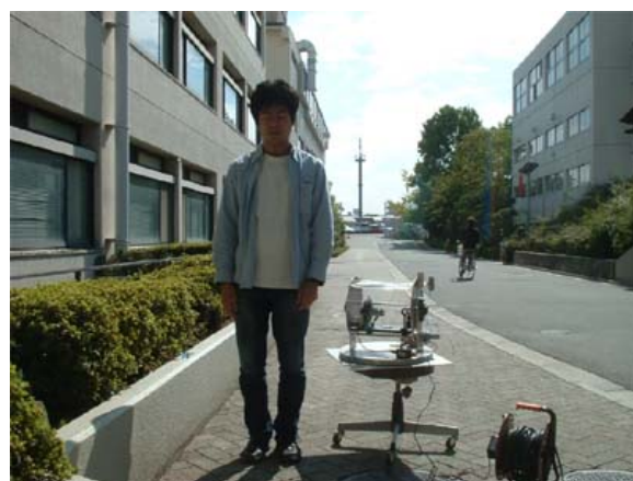
Fig.3 Apparatus, which produces metal nanoparticles from metal oxides using solar-pumped pulse laser.
