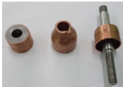
(d) Job: Cu tube to soft iron disc welding & free forming
