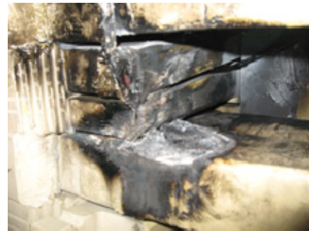
Figure 1 Endwinding stator insulation breakdown in water-cooled generators
