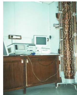
Fig. 4.2.1 Impulse fault analysis set-up with analog model of transformer winding
