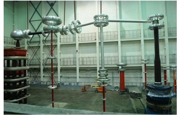
Fig. 4 The 1100 kV extra high voltage bushing designed and manufactured by China XD Group and Xi'an Jiaotong University [25, 26].
