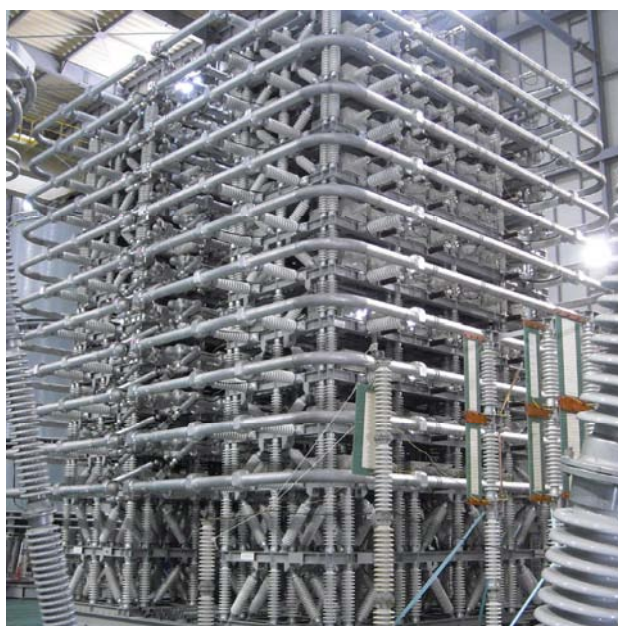
Capacitor bank of adjusting the transient recovery voltage. (Provided by Hitachi, Ltd. Power Systems Company)
