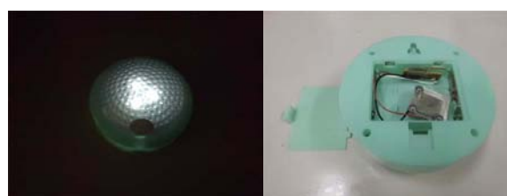
Fig.5 LED illumination using air cell.
