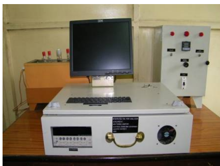
Fig. 4.4.1.1 Developed PDC-RVM Analyzer
