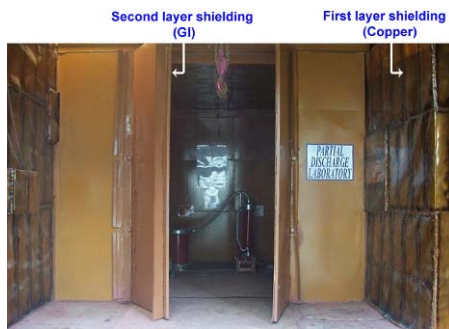
Fig. 4.3.1 Double Shielded Partial Discharge Laboratory
