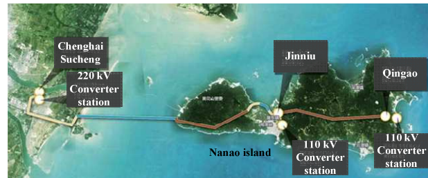
Figure 4. Geographic and electrical connection graph of Nanao island three terminal HVDC flexible transmission system
