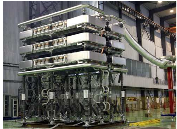
Figure 2. The converter valve tower of HVDC flexible transmission
