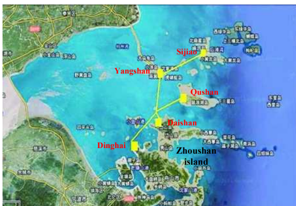
Figure 3. Geographic and electrical connection graph of Zhoushan island five terminal HVDC flexible transmission system
