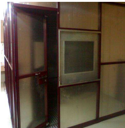
Fig. 2 Faraday Cage (4 m x 5.7 m x 3 m)
