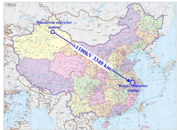
Figure 2 Zhundong-Wannan \pm 1100\text{kV} UHV DC transmission project
