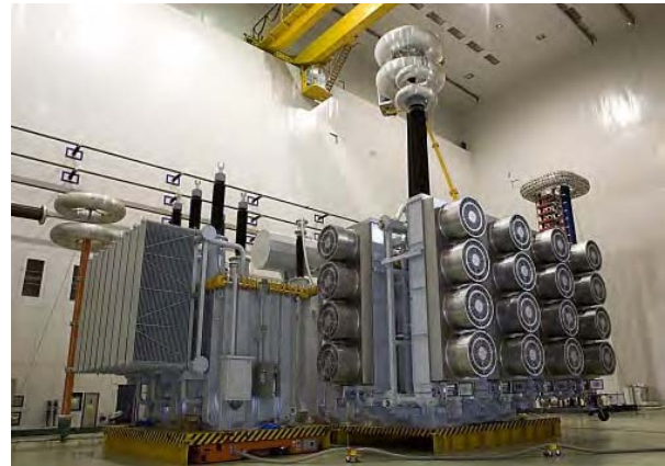
Figure 4 1000kV/1000MVA UHV step-up transformer
