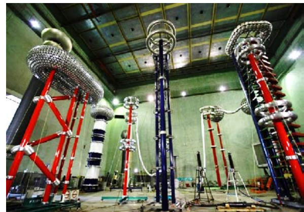
Figure 2. Type test for \pm 320 kV extruded HVDC cable in Zhoushan, China.
