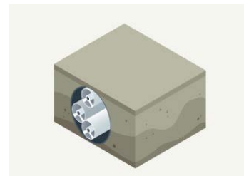
Figure 4. Tunnel installation of Su-tong GIL [6]
