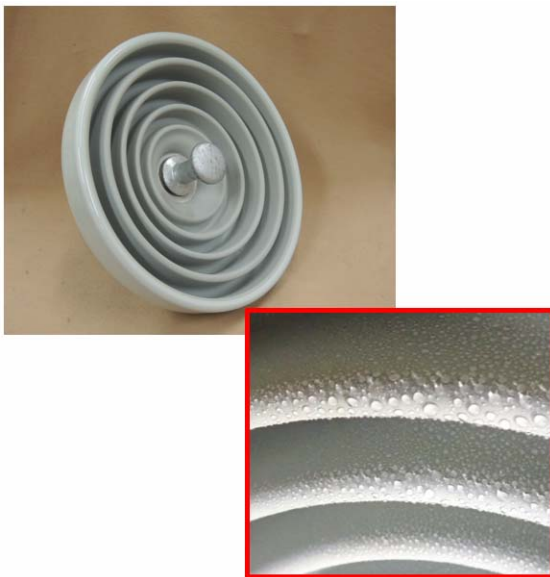
Fig. 1. RTV coated insulator
