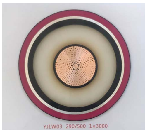
Fig. 2. \pm 500 kV XLPE cable with 3000 mm 2 section [6]
