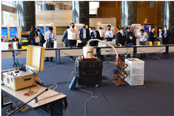
Fig. 6. Testing transformer and PD source in demo-session.
