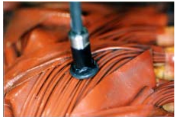
Fig. 2. The optical probe on the coil surface of an induction motor
